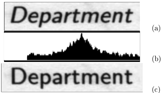
Fig. 5: (a) A word with slant characters (grey level image); (b) The gradient orientation histogram; (c) Slant corrected text (slant angle obtained is 12.04 degrees).
