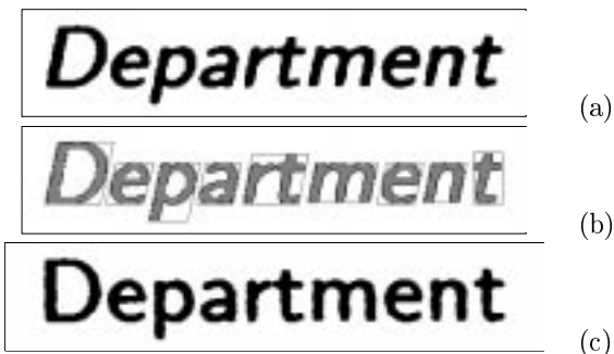
Fig. 6: (a) A word with slant characters; (b) Parallelograms fitted to the characters (connected components); (c) Slant corrected text (slant angle is 12.0 degrees).
