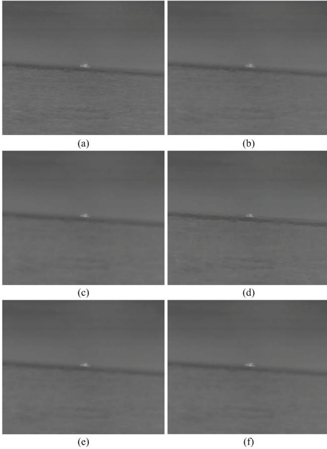
Fig. 5. Comparison results of IR image with low contrast. (a) The original IR image; (b) The result of anisotropic diffusion filtering ( $num_{iter} = 10, t = 15$ ); (c) The result of bilateral filtering ( $w=9; \sigma=[5, 0.05]$ ); (d) The result of Kuwahara filtering ( $L=3$ ); (e) The result of mean shift filtering with fixed range bandwidth ( $h_r=15$ ); (f) The result of the proposed method.
