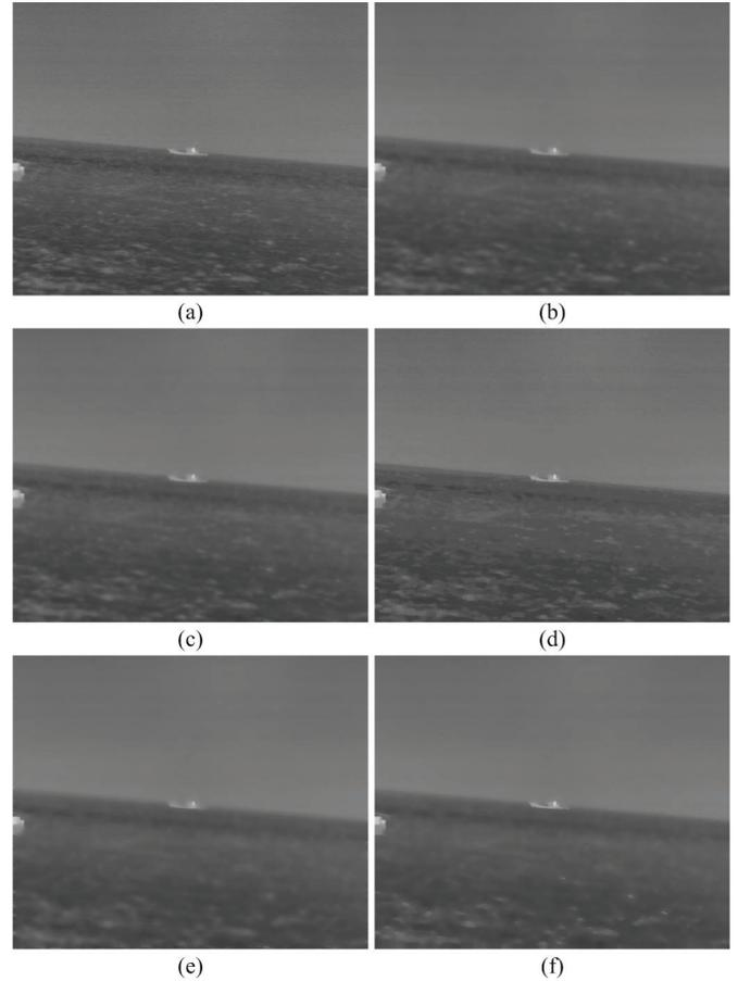
Fig. 4. Comparison results of IR image with complex sea clutters. (a) The original IR image; (b) The result of anisotropic diffusion filtering ( $num_{iter}=15$ ,  $t=10$ ); (c) The result of bilateral filtering ( $w=5$ ;  $\sigma=[3, 0.1]$ ); (d) The result of Kuwahara filtering ( $L=1$ ); (e) The result of mean shift filtering with fixed range bandwidth ( $h_r=35$ ); (f) The result of the proposed method.
