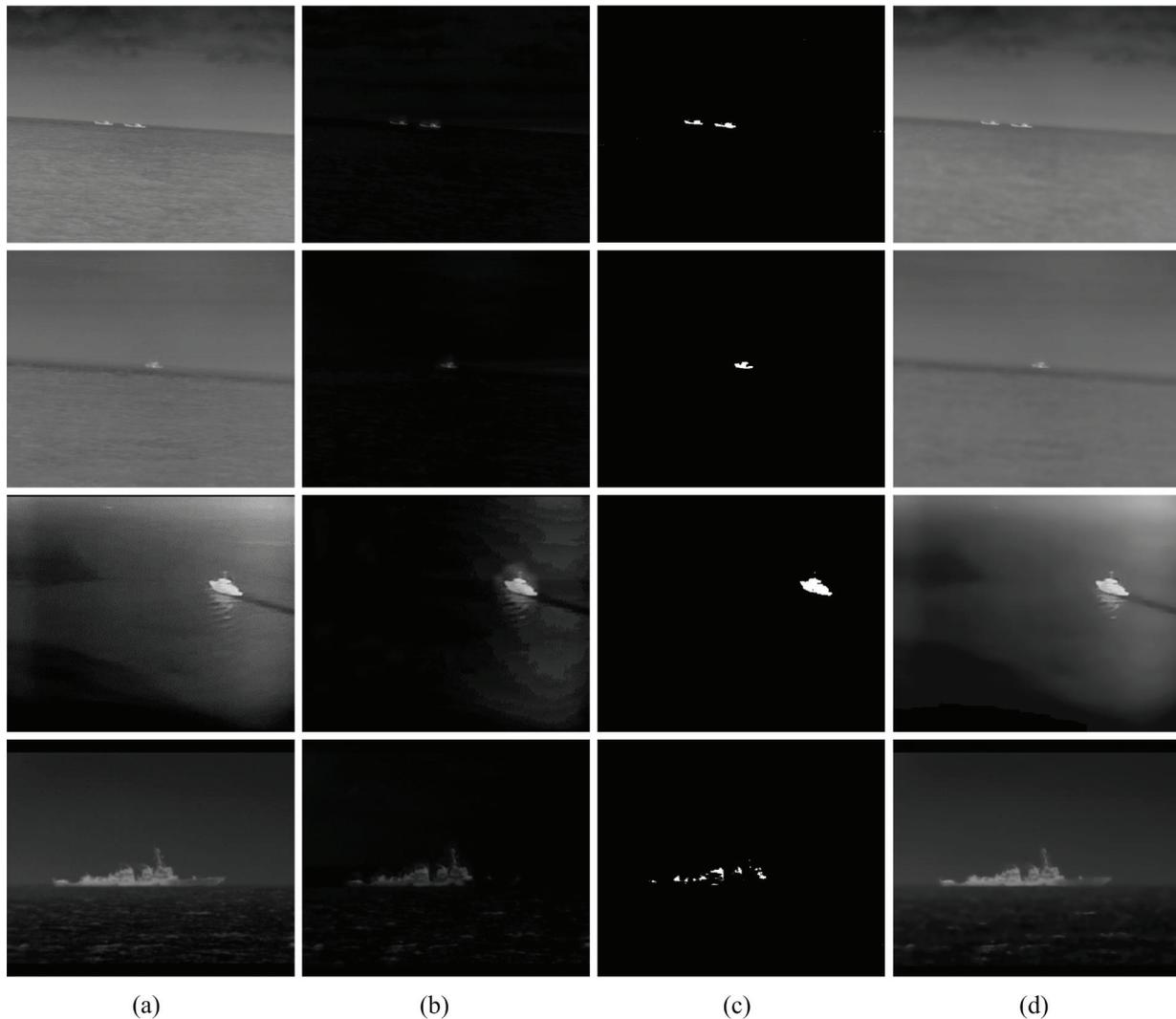
Fig. 3. Image smoothing result. (a) The original IR image; (b) The salient region map; (c) The binarized mask; (d) The smoothed image.
