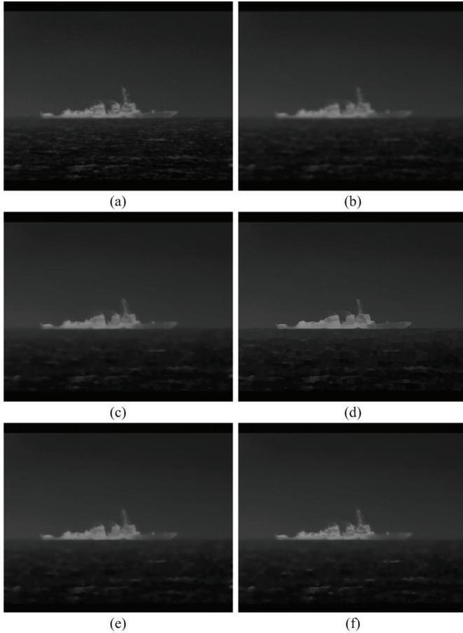
Fig. 7. Comparison results of IR image with uneven ship target. (a) The original IR image; (b) The result of anisotropic diffusion filtering ( $num_{iter}=15, t=15$ ); (c) The result of bilateral filtering ( $w=9; \sigma=[5, 0.05]$ ); (d) The result of Kuwahara filtering ( $L=3$ ); (e) The result of mean shift filtering with fixed range bandwidth ( $h_r=20$ ); (f) The result of the proposed method.
