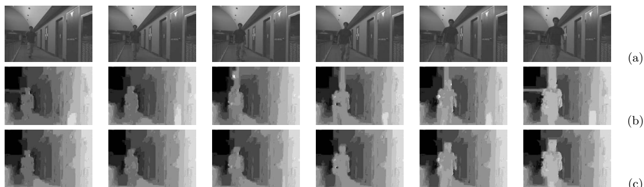
Figure 2. (a) A set of left input images from a stereo image sequence. (b) The disparity map computed without temporal coherence. (c) The disparity map computed using both spatial and temporal regularity.
