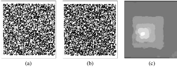
Fig. 3: The matching result for Random Dot Stereograms. (a) left image; (b) right image; and (c) the 3D surface recovered.
