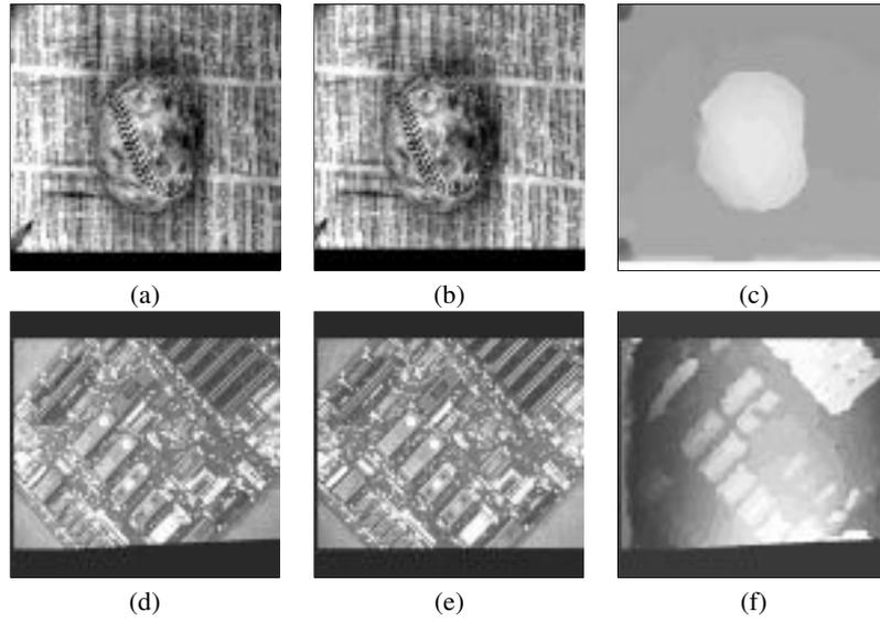
Fig. 5: The matching result for some close range images. (a,d) left image; (b,e) right image; and (c,f) the 3D surface recovered.
