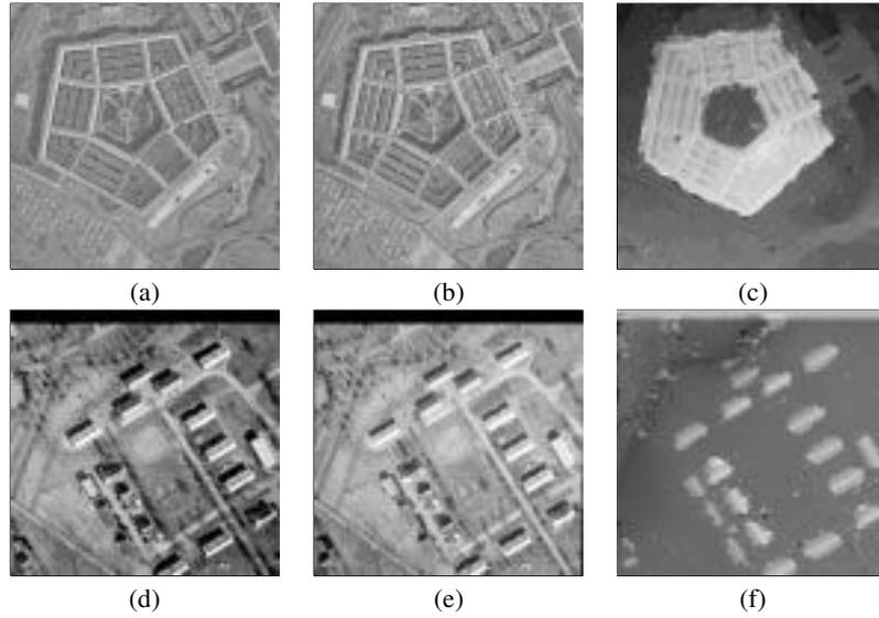
Fig. 6: The matching result for some aerial photo images. (a,d) left image; (b,e) right image; and (c,f) the 3D surface recovered.
