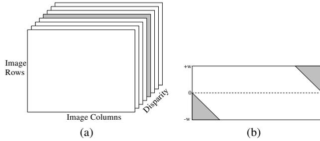
Fig. 1: (a) An illustration of the correlation matrix. (b) One horizontal slice of the correlation matrix in (a).
