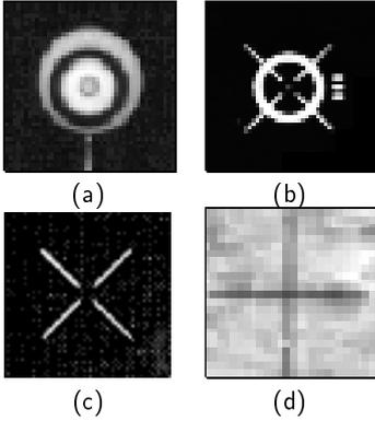
Figure 2: Illustration of several typical shapes of fiducial mark in an aerial photo image.
