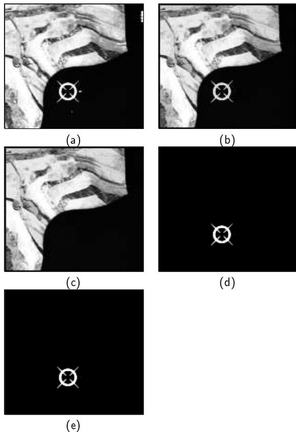
Figure 3: The process of the automated segmentation of fiducial marks. (a) one of the original sub-images containing a fiducial mark; (b) morphology opening by area 100; (c) morphology opening by aspect ratio 1.2; (d) subtraction of image in (c) from the image in (b); and (e) the brightest object by using morphological reconstruction.
