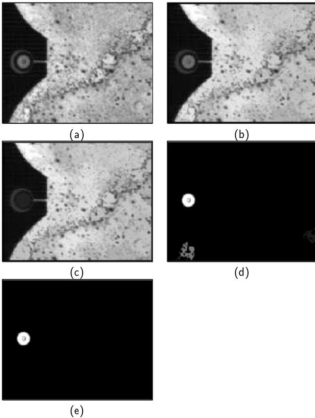
Figure 5: The process of the automated segmentation of fiducial marks for a different image. (a) one of the original sub-images containing a fiducial mark; (b) morphology opening by area 100; (c) morphology opening by aspect ratio 1.2; (d) subtraction of image in (c) from the image in (b); and (e) the brightest object by using morphological reconstruction.
