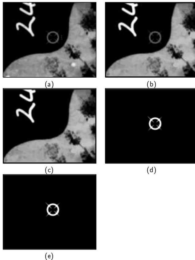
Figure 4: The process of the automated segmentation of fiducial marks for a different image (with letters). (a) one of the original sub-images containing a fiducial mark; (b) morphology opening by area 100; (c) morphology opening by aspect ratio 1.2; (d) subtraction of image in (c) from the image in (b); and (e) the brightest object by using morphological reconstruction.
