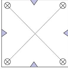
Figure 1: Illustration of the location of the fiducial marks and principal point for an aerial photo image. The intersection of the dotted line indicates the principle point.
