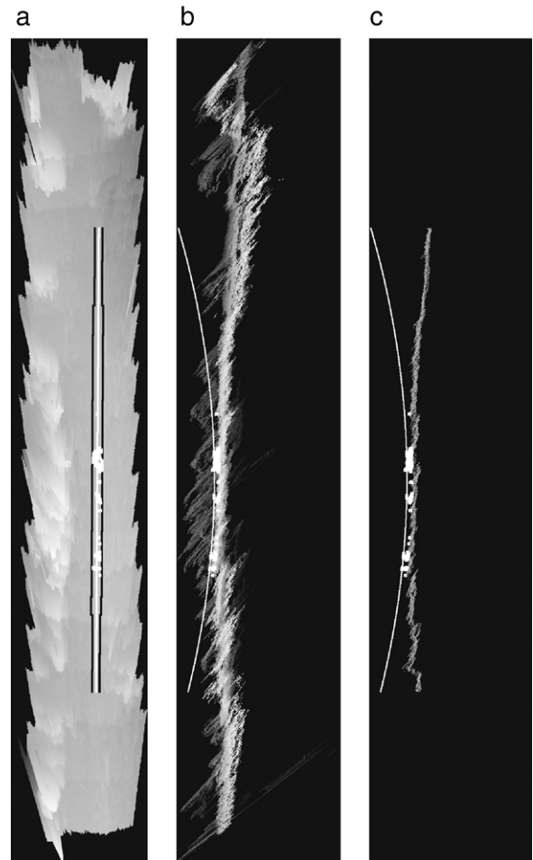
Fig. 11. (a) Top view of a powerline (with envelope) suspended on 2 power poles over a landscape. (b) Side view of a powerline and all objects in the landscape. (c) Side view of a powerline and objects within the catenary envelope (powerline sagging in (b) and (c) has been magnified). Powerline represented as white pixels. The gray level intensities are proportional to the height of each pixel in the landscape. The catenary envelope is represented by black pixels, and vegetation found within the catenary envelope is represented by white blobs.
